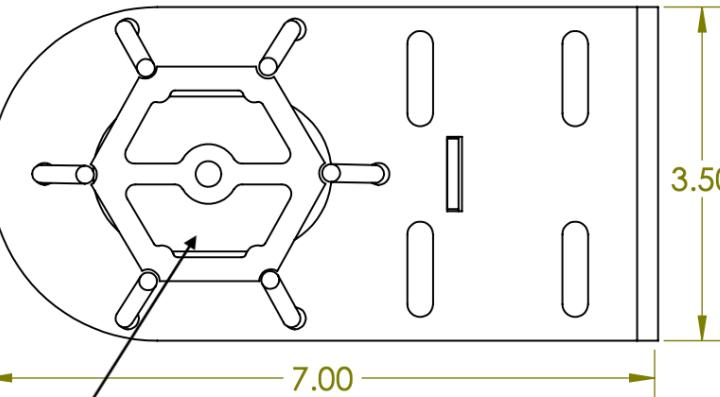
Maximum fitting diameter is 1.6" for base plate opening
