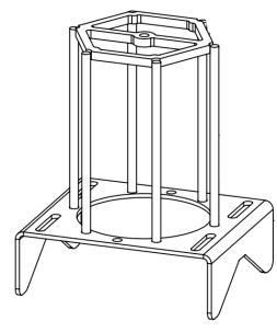
The SG511 ESFR Inline guard is designed for ESFR fire sprinkler heads. This guard uses the SG905 SprinkLOCK plate to secure the guard around the line fitting. If your application is an ESFR on an end of line fitting, please refer to the SG331 ESFR ADACAP or SG512 End of Line ESFR
